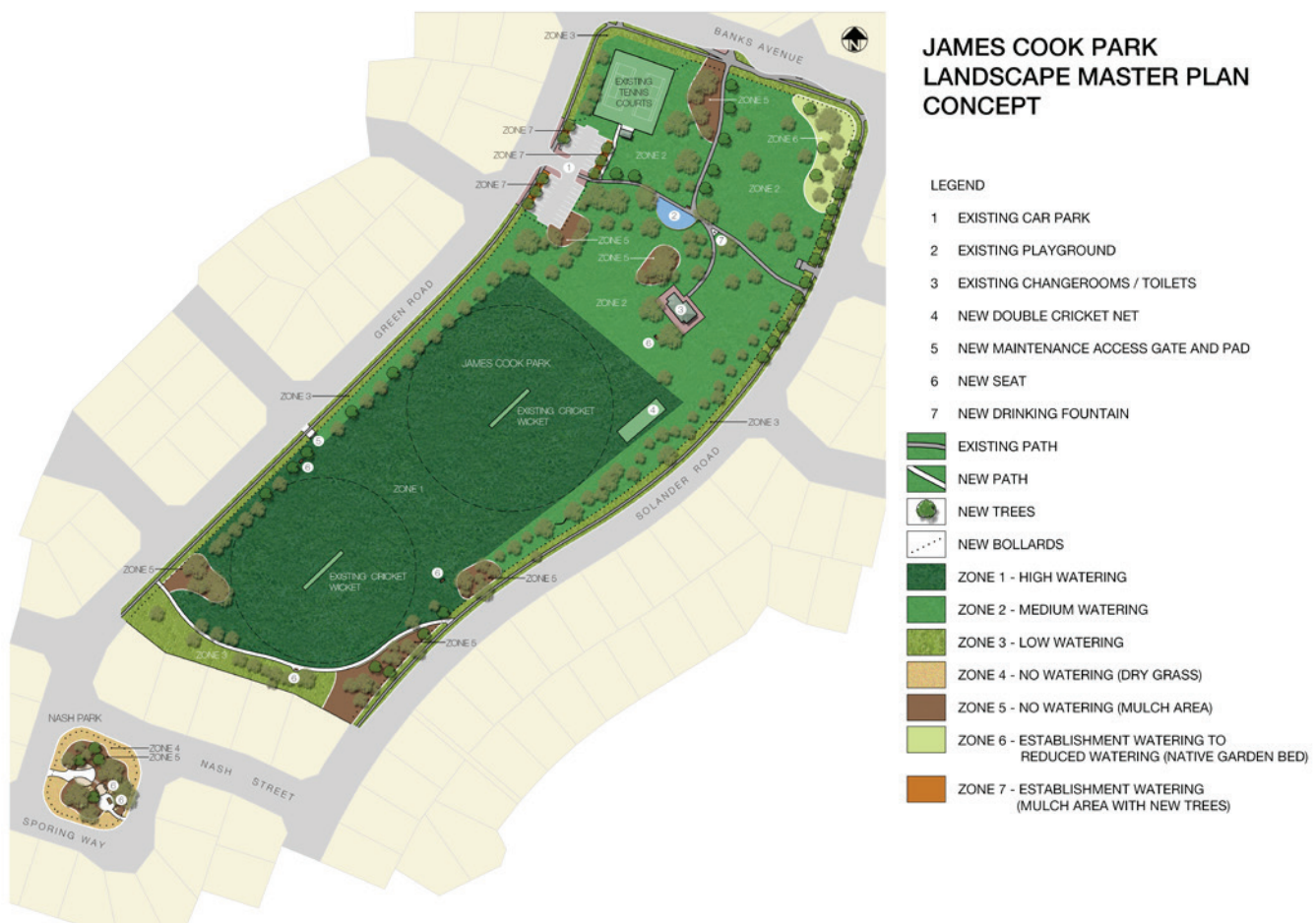
Figure 1: Concept Map of Proposed Irrigation Works and Upgrades at James Cook Park, Hillarys (including Nash Park)
