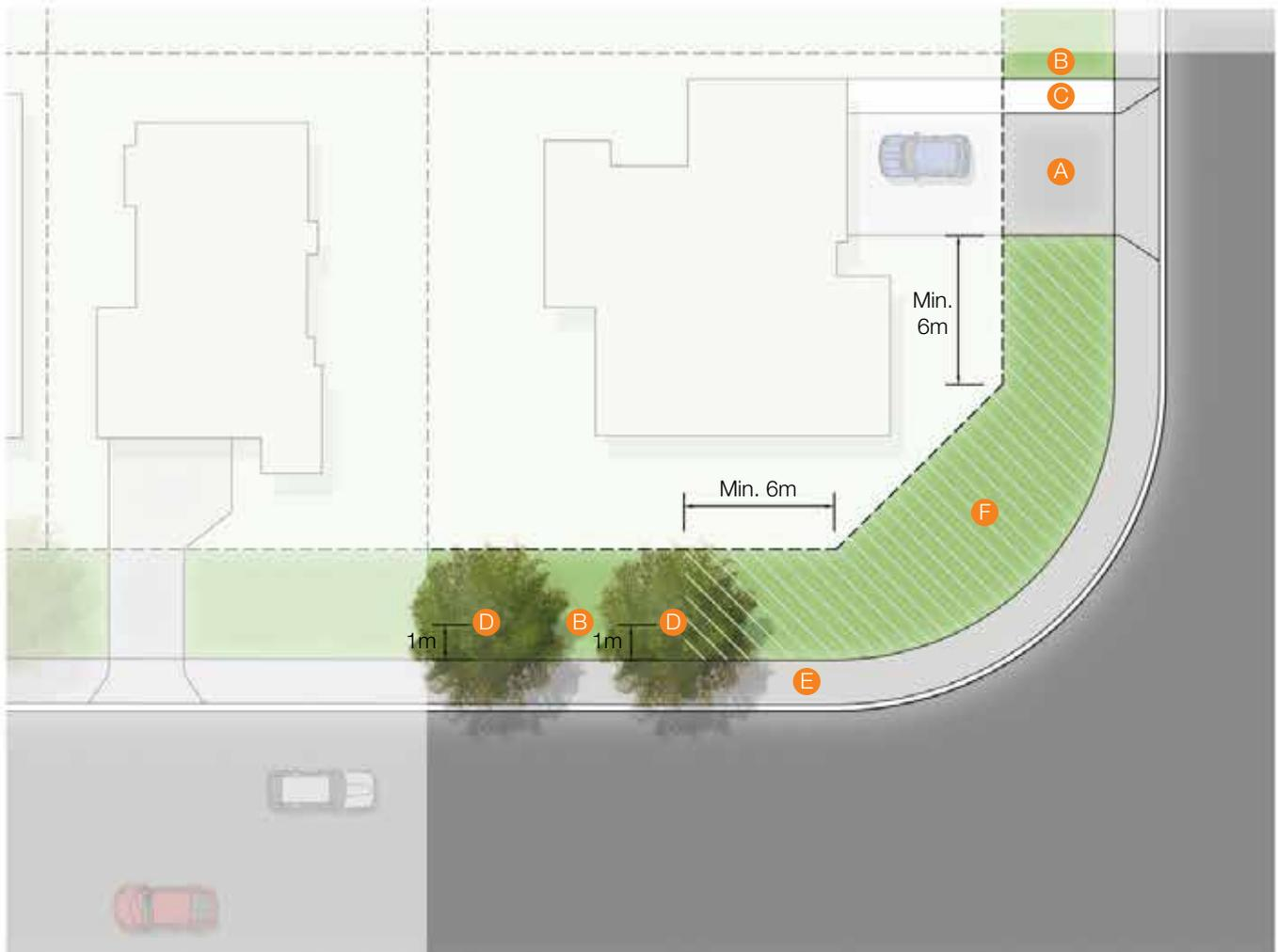
**FIGURE 4:** Typical corner verge layout with footpath
