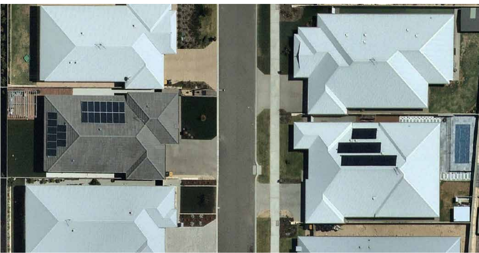
FIGURE 5: Crossovers constructed with continuous footpaths.
