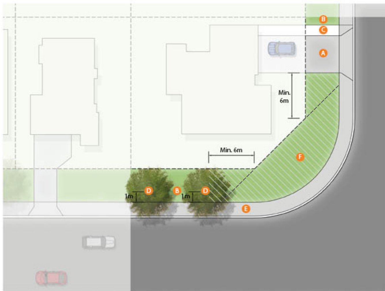
FIGURE 4: Typical corner verge layout with footpath
