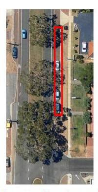
Figure 5: Extent of on-street parking to be removed to achieve SISD
