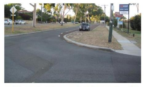
Figure 4: Example of parked vehicle obstructing SISD at the existing northern driveway
