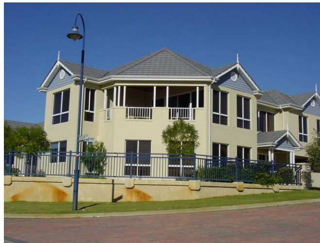
Photo 3: Good example of address both streets and use of open style fencing
