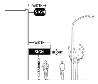
NOTE: Clearance is measured from the finished ground level to the sign directly above.
