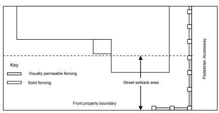
Figure 4. Fencing adjacent pedestrian accessway
