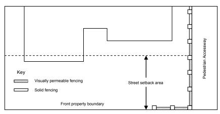
Figure 5. Fencing adjacent pedestrian accessway
