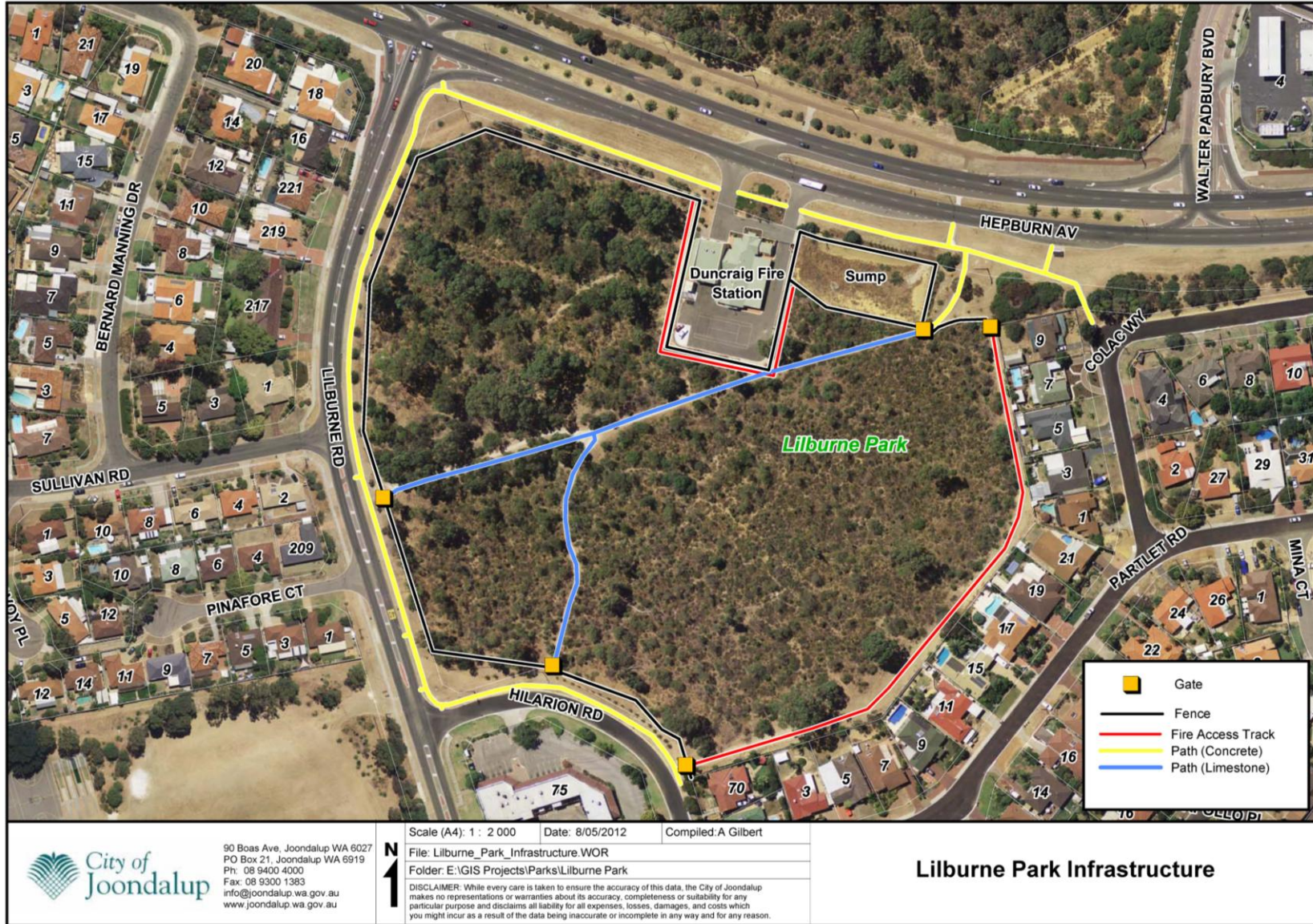
Figure 23: Infrastructure at Lilburne Park
