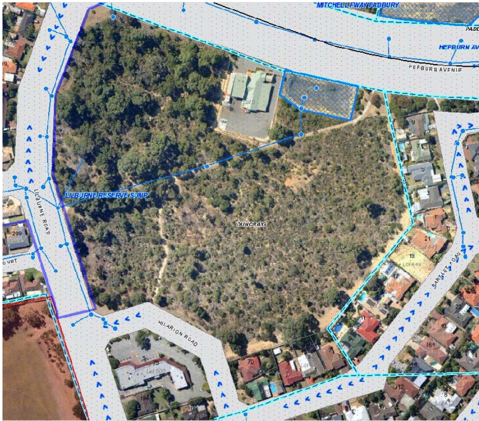
Figure 8: Lilburne Park Drainage Lines and Sump
