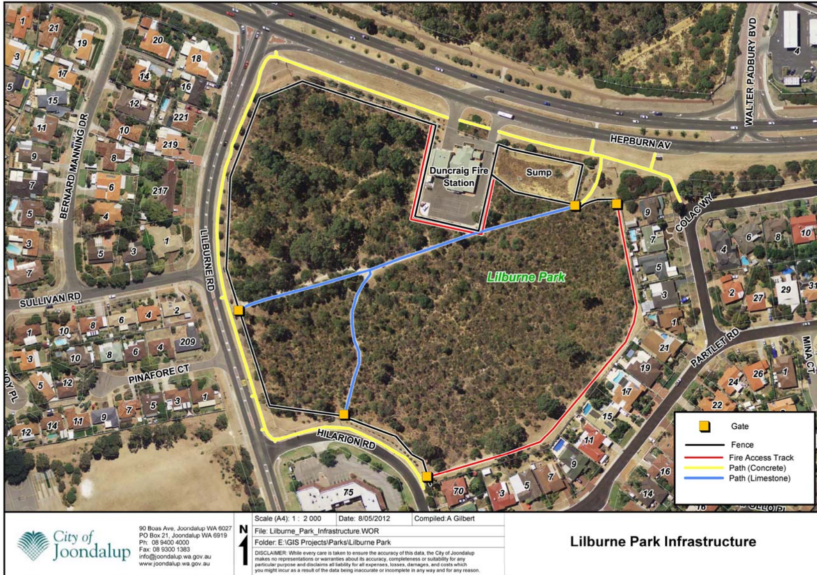
Figure 23: Infrastructure at Lilburne Park
