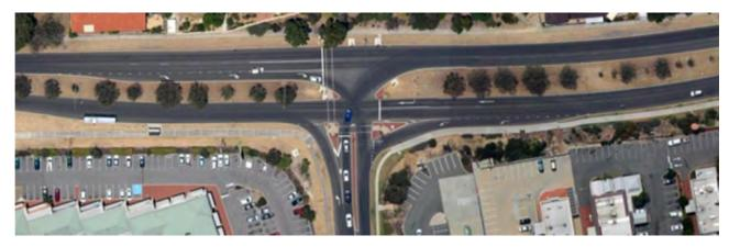
Whitfords Avenue/Dampier Avenue/shopping centre access – A 4-way signalised intersection including left and right turning pockets on Whitfords Avenue as shown in Figure 5-8. Provision for crossing pedestrians is explicitly included within the signal phasing.
