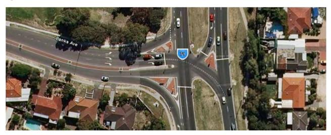
Marmion Avenue/Cook Avenue – A 3-way priority controlled intersection including a right turning pocket and left turn slip lane on Marmion Avenue, as shown in Figure 5-11. The seagull island within the central median allows for staged crossing for right-turning traffic, with sufficient space for queuing of up to two cars. This significantly improves traffic operations for right-turning vehicle movements.
