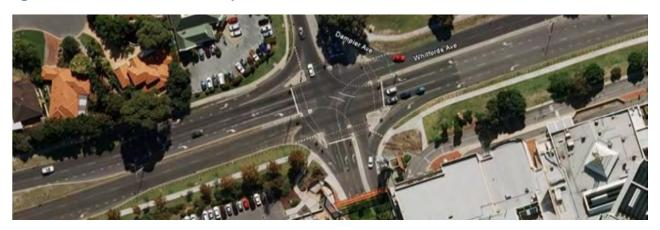
Whitfords Avenue/Marmion Avenue – A major 4-way signalised intersection including right turning pockets and left-turn unsignalised slip lanes on all approaches. The existing layout of this intersection is shown in Figure 5-9. Pedestrian provision has not been explicitly included within the signal phasing; however actuated crossing facilities are provided. Long red phases for all approaches provide sufficient crossing time for pedestrians intending to cross at this location.
