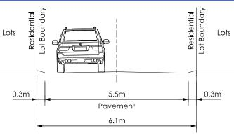
TYPICAL ROAD CROSS SECTIONS Camberwarra Primary School Structure Plan
