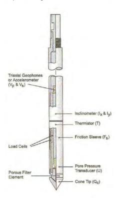
Figure 1: Cone Diagram
