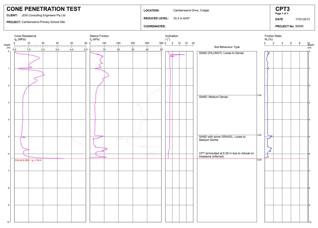
REMARKS: \* Surface level interpolated from survey plan provided by the client. File: P:\82006 Craigie, Camberwarra Primary School Site\Field\CPT3.CP5 Cone ID: Probedrill Type: EC04
