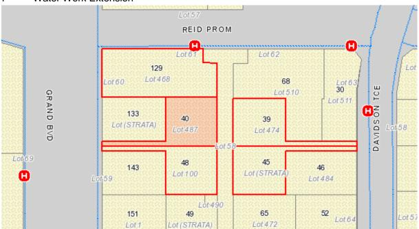
A water extension will be required from Reid Promenade to the Central Walk intersection, which is a distance of 70 metres. It is estimated that an all-in cost for a water main extension is \$300 per metre at a total cost of \$21,000. This work would be undertaken by an external contractor.
