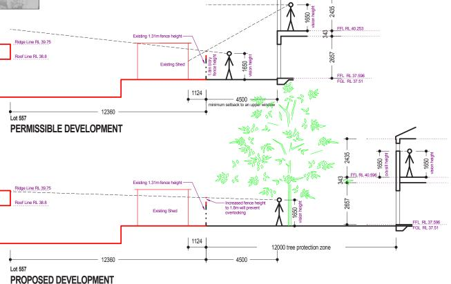
FIGURE 17: EXISTING RESIDENTIAL INTERFACE - SECTION B
