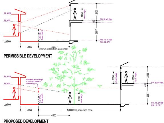
FIGURE 16: EXISTING RESIDENTIAL INTERFACE - SECTION A
