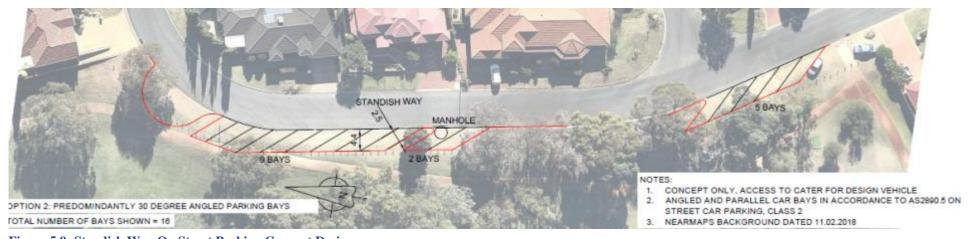
Figure 5.9: Standish Way On Street Parking Concept Design
