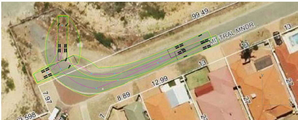
Figure 6 Swept path of 3 point turn of 12.5m truck
