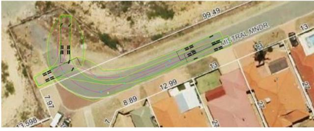
Figure 5-1 Swept Path (3-point turn – 12.5m truck)
