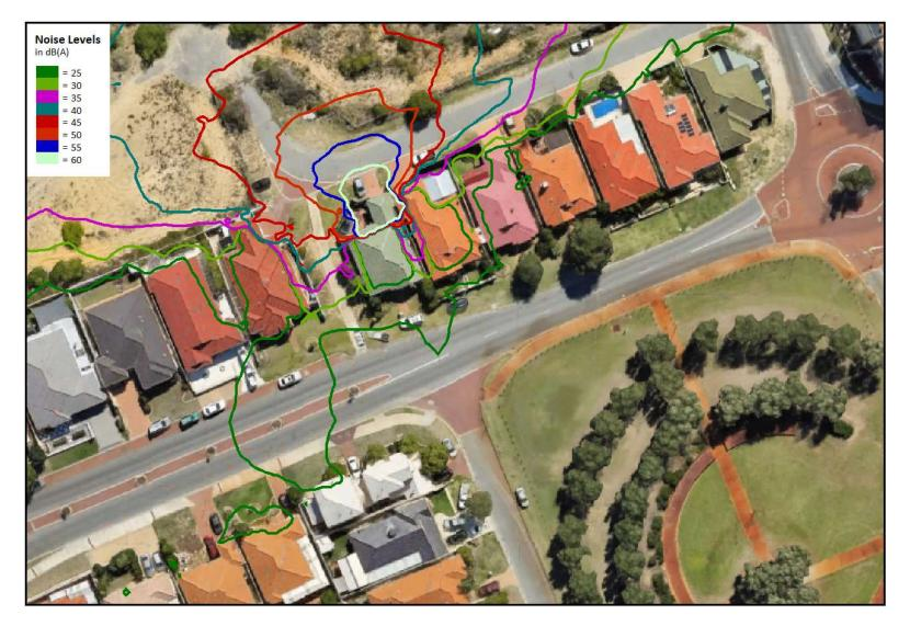
Figure 9: Worst-case noise level contour for scenario 4.
