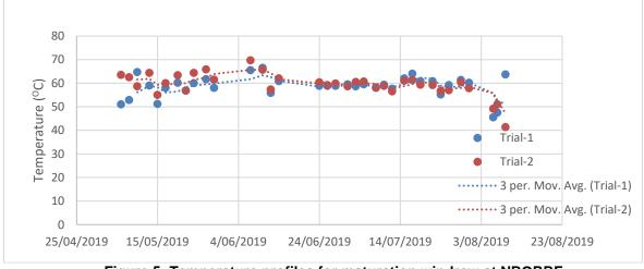
Figure 5: Temperature profiles for maturation windrow at NBORRF
