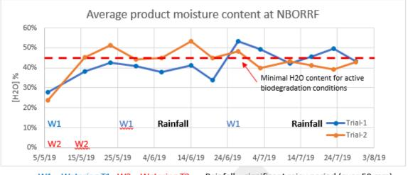
W1 = Watering T1 W2 = Watering T2 Rainfall = significant rainy period (over 50 mm)
