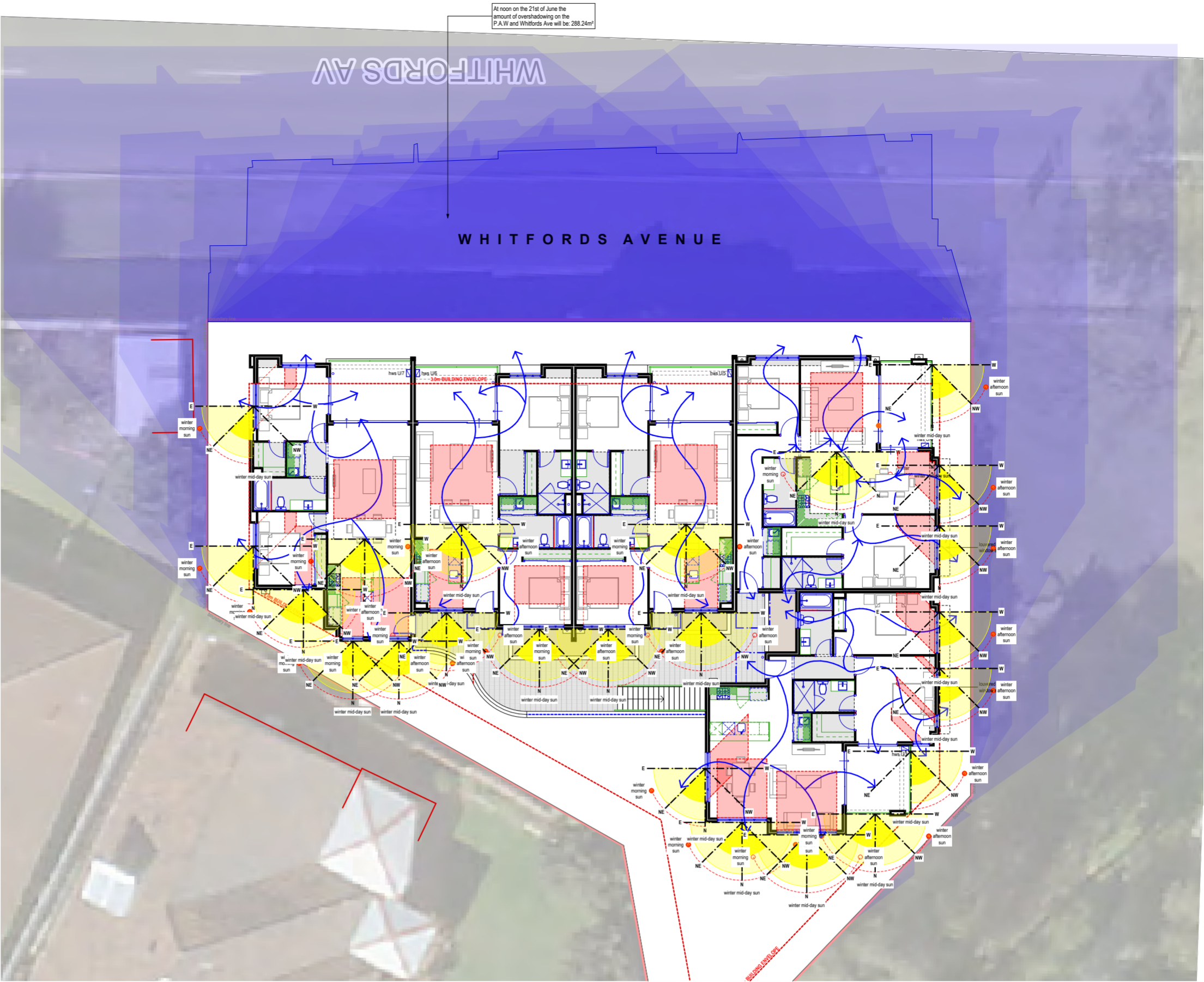
Sun Study & Ventilation Diagram (Upper Floor) scale1:200
