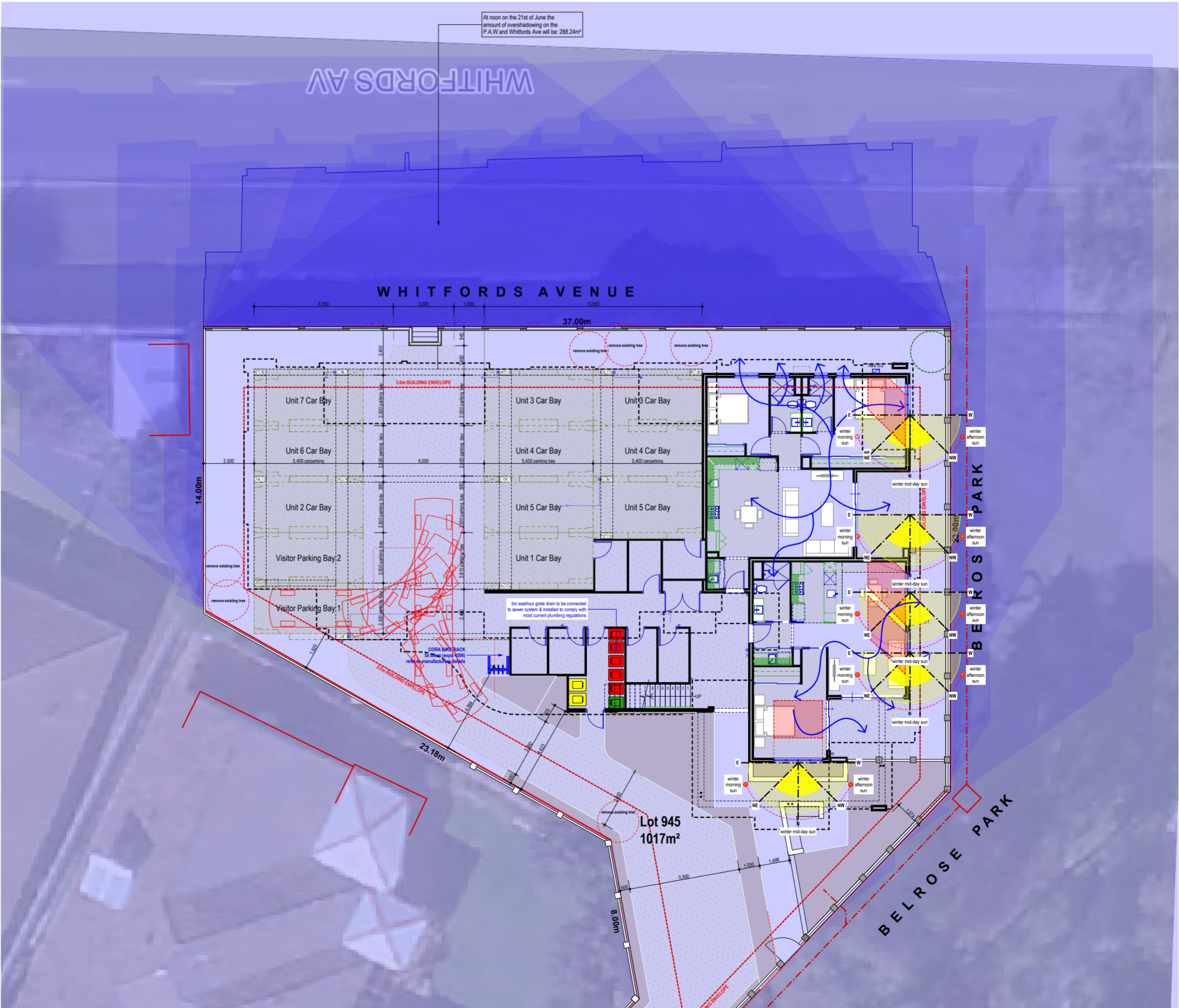
Sun Study & Ventilation Diagram (Ground Floor) scale1:200
