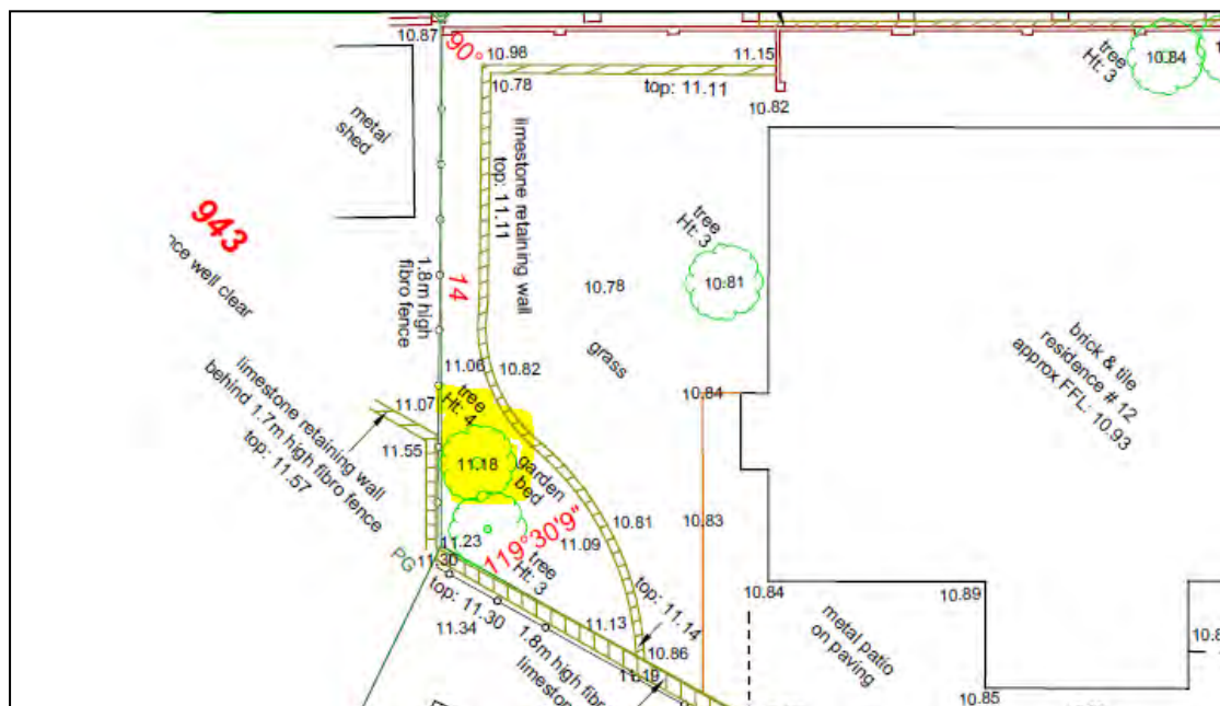
Figure 2 - Extract of feature and contour survey plan
