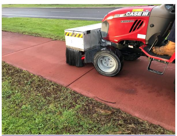
Figure 14: WeedSeeker Technology in use on a footpath
