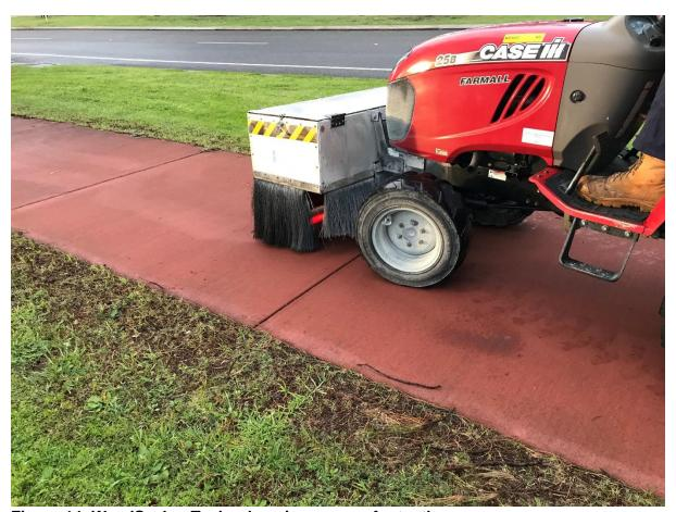
Figure 14: WeedSeeker Technology in use on a footpath
