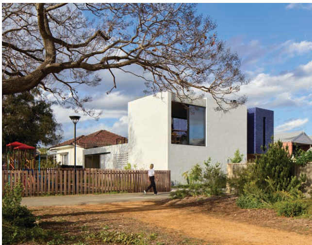
Photo G3.9a This dwelling designed to reduce the impact of development overshadowing primary garden area of adjoining lot (PC)
