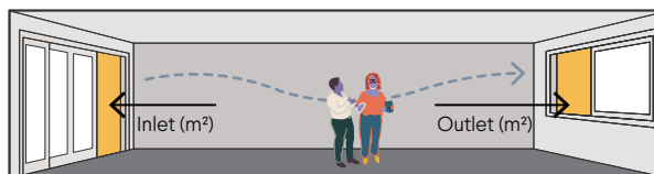
Figure G2.2a Natural ventilation for passive cooling
