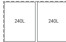
2-bin system Minimum depth - 0.74m Minimum length - 1.16m Minimum area - 0.86sqm
