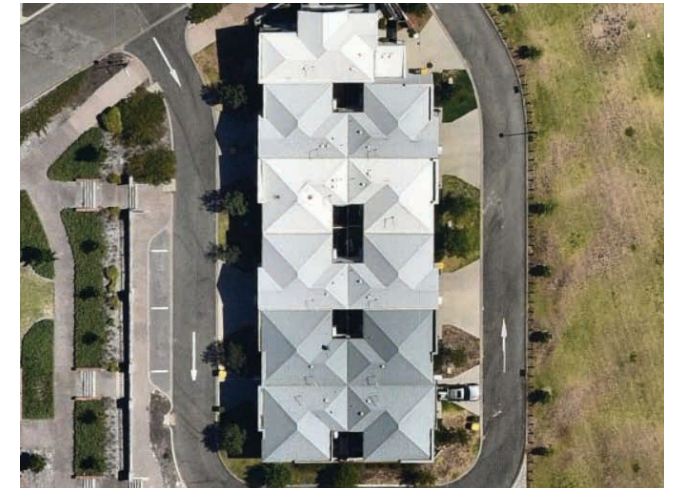
Photo G2.10b Consolidated vehicle access points reduce crossovers to the street and allow for street parking
