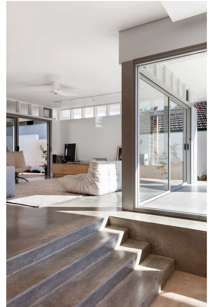
Photo G2.2c Orienting windows to the north provides effective winter passive heating to primary living spaces (PC)
