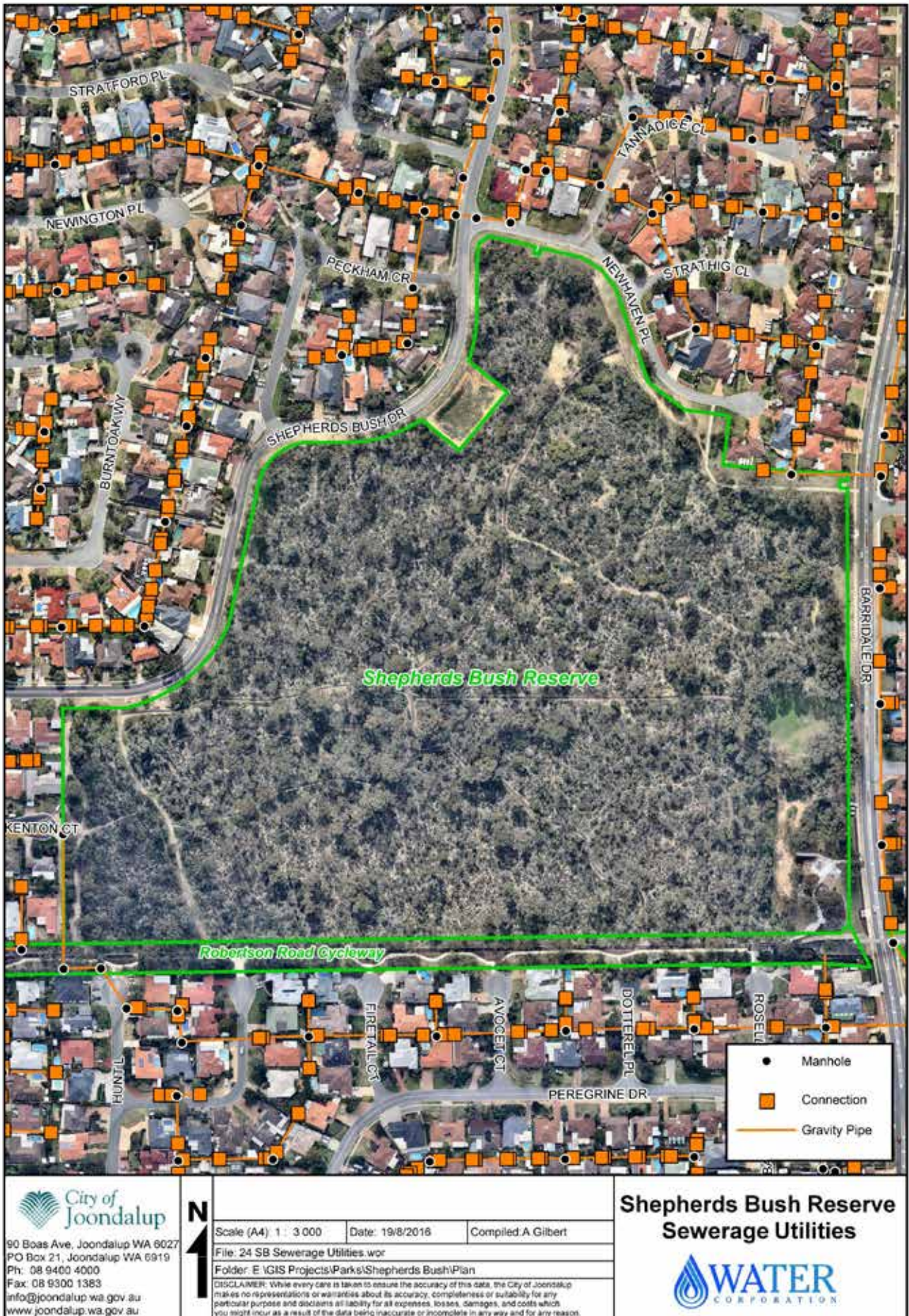
Figure 24: Shepherds Bush Reserve Sewerage Utilities
