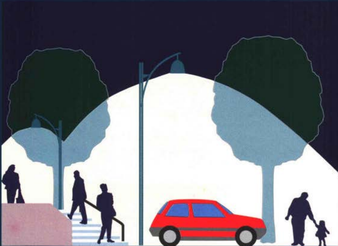
C4.6 Provide illumination particularly at hazards such as steps
