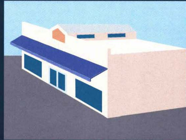
■ B3.4 Screening of rooftop services designed as an integral part of the building
