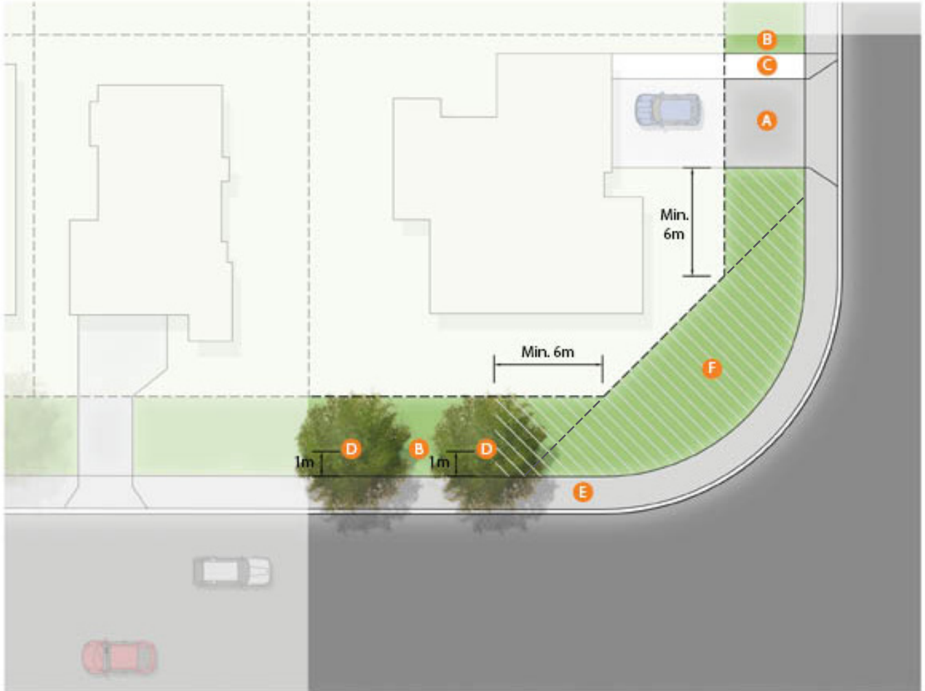
FIGURE 4: Typical corner verge layout with footpath
