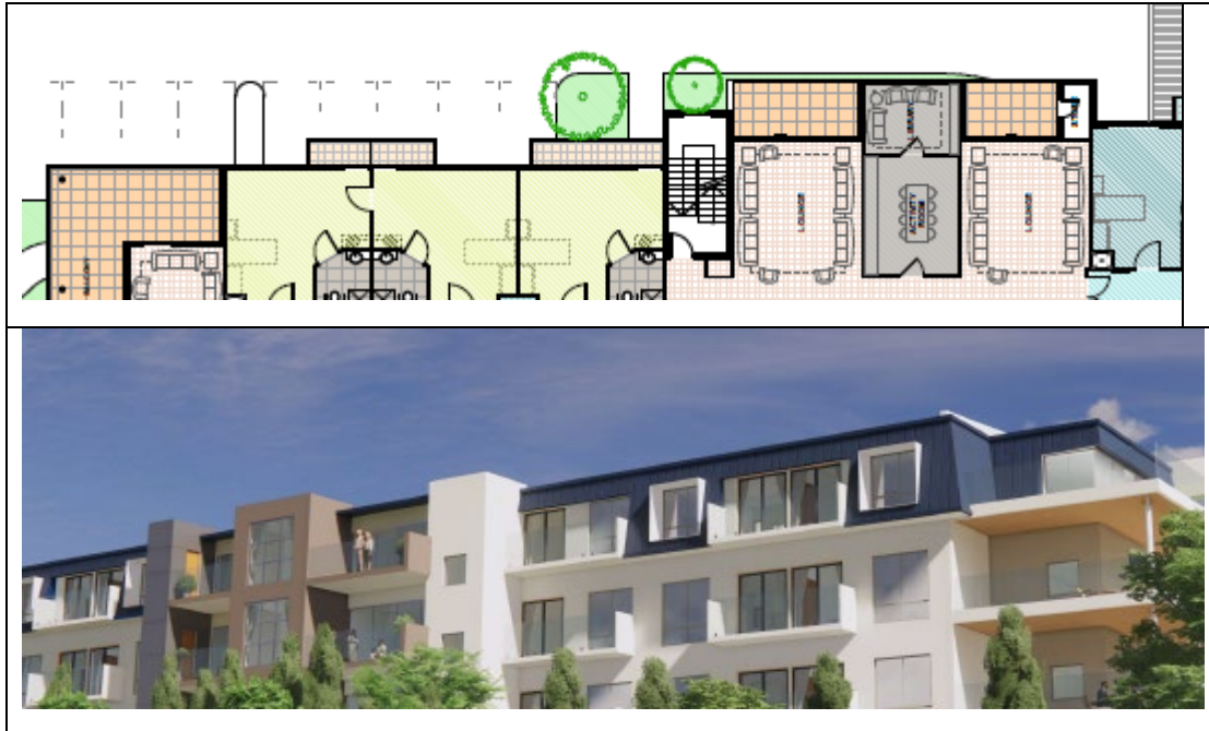
Figure 3 – Recessive Wall and Setback Treatments to break the horizontal massing and building which increase as topography changes result in increased building height
