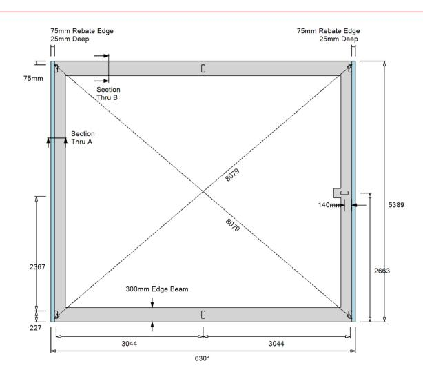
For more information please refer: Construction Footing Report Stratco 15 Degrees Gable Roof Shed Class 1A & Class 10 Buildings 50098. Please note that the internal concrete beams are not shown on the above layout and it is the builders responsibility to select the appropriate design scenario based on the soil conditions on site and Drawing No. 50098-6-ST-100 from the report.
