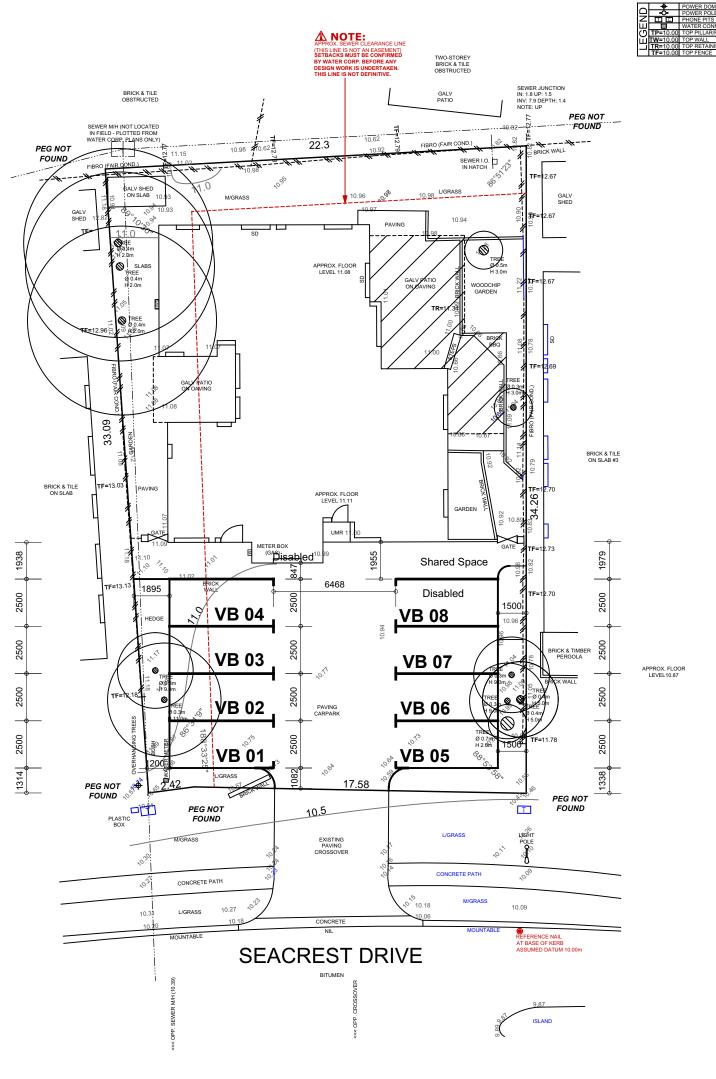
Survey shows visible features only and will not show locations of underground pipes or conduits for internal or mains services. Verification of the location of all internal and mains services should be confirmed prior to finalisation of any design work.
