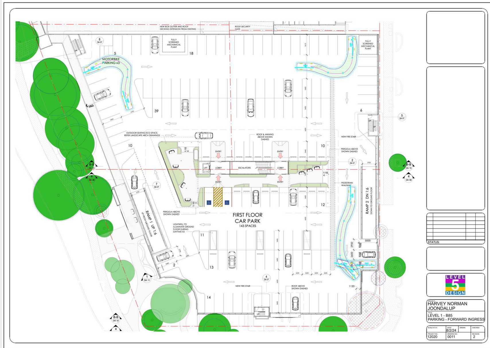
Figure E11 – Swept Path – Ground – B85 Parking – Forward Ingress
